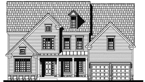
Front Elevation Number 4 Shown with Standard Siding, Optional Stone Water table, and Optional Dormers
