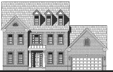
Front Elevation Number 1 Shown with Optional Full Brick and Optional Dormers
